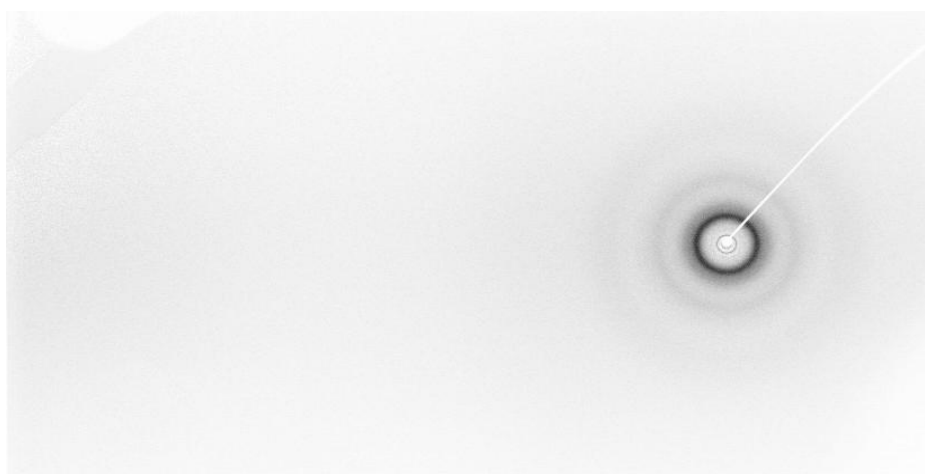
Figure 2.7 Two-dimensional scattering pattern of V-ITZ sample, obtained using the laboratory diffractometer.
