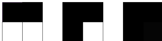
Fig. 4.34 Three different kinds of defects occurring in the FK configurations defined as deviations from the checkerboard pattern. The black and white cells indicate either the presence or absence of an ion at the lattice site.
