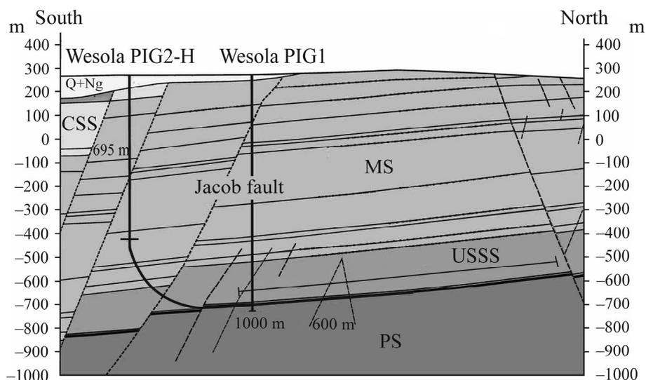
**Fig. 4.** Boreholes drilled to the 501–510 coal seams: CSS—Cracow sandstone series; MS—mudstone series; PS—paralic series; USSS—Upper Silesia sandstone series.
