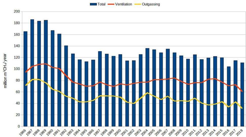
**Fig. 11** The Pniówek mine-specific methane emission (JSW—internal reports)
