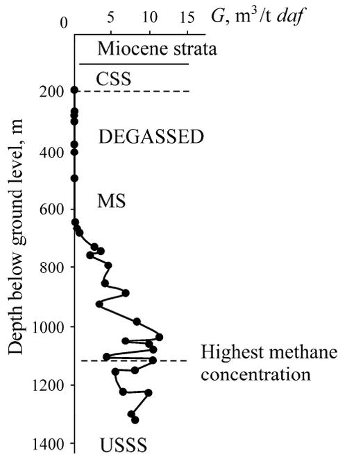
Fig. 3. Methane distribution in the LG-23 borehole: CSS—Cracow sandstone series; MS—mudstone series; USSS—Upper Silesia Sandstone Series.
