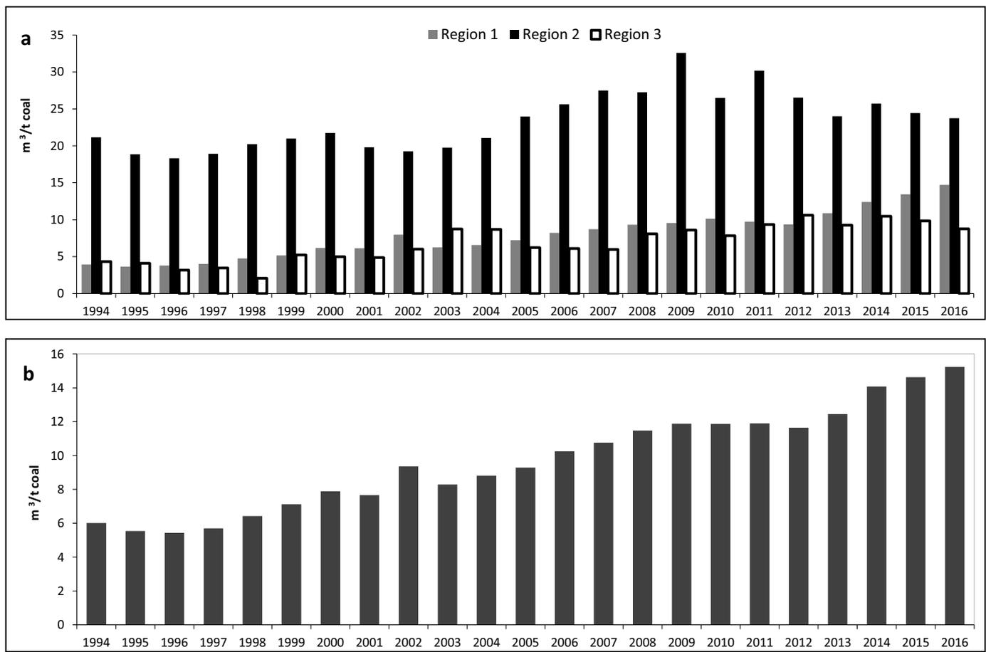
Fig. 6. Specific methane emissions in three USCB regions (a) and in the USCB as a whole (b).
