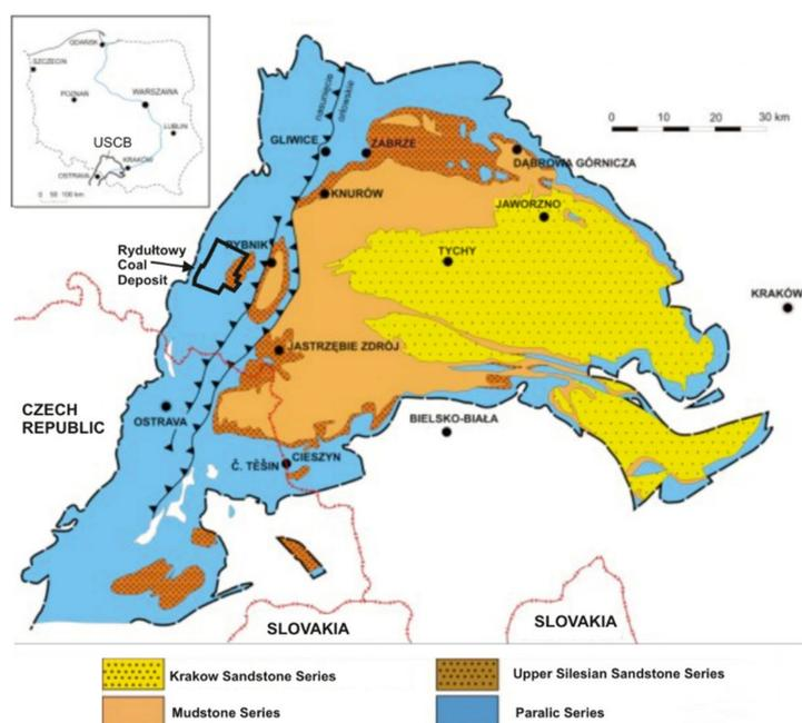
**Figure 1.** The Rydułtowy coal deposit against the background of the lithology and stratigraphy of the Upper Silesian Coal Basin.
