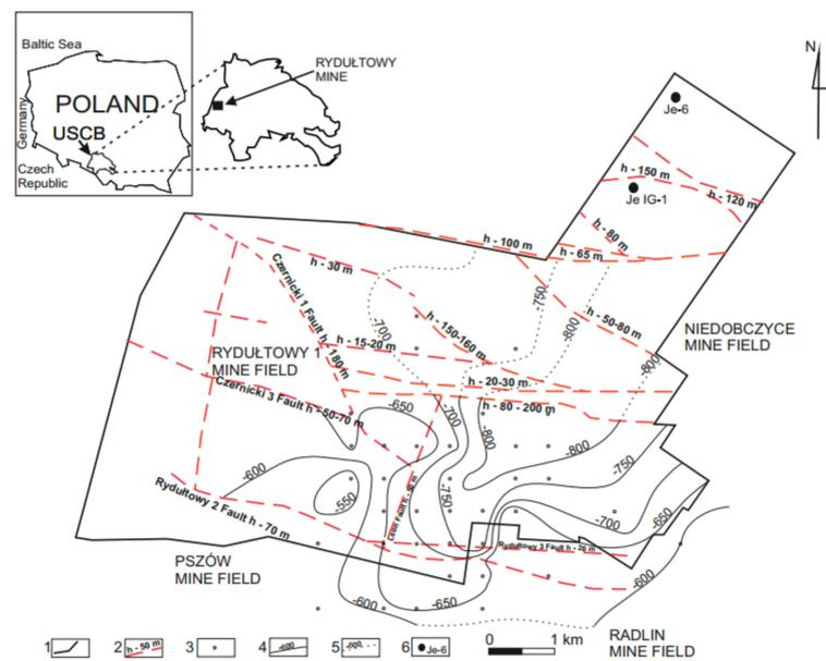
**Figure 3.** Top of the methane seams with  $G > 4.5 \text{ m}^3/\text{Mg}$  coal daf against the background of the tectonics of the research area (modified after Rydułtowy mine archive materials): 1—boundary of the Rydułtowy mine field, 2—fault with the displacement value, 3—estimation point of the top of the methane seams, 4—line of the top of the methane seams (m above sea level), 5—presumed line of the top of the methane seams, 6—surface bore hole.
