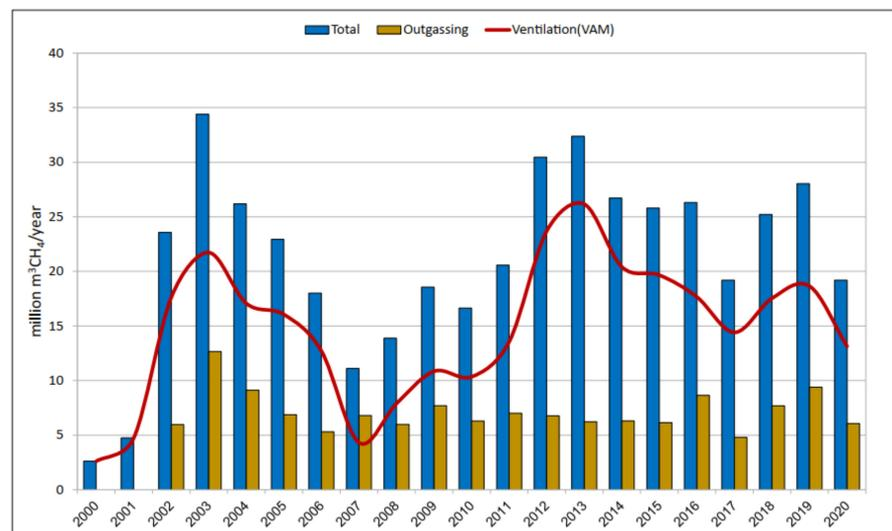
Figure 9. Total methane emissions and outgassing and ventilation air methane from 2000–2020 in the Rydułtowy mine.
