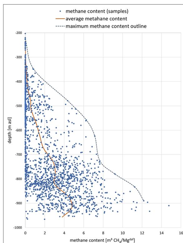
**Figure 2.** Depth distribution of the methane content in the Rydułtowy mine (Rydułtowy mine archive materials).
