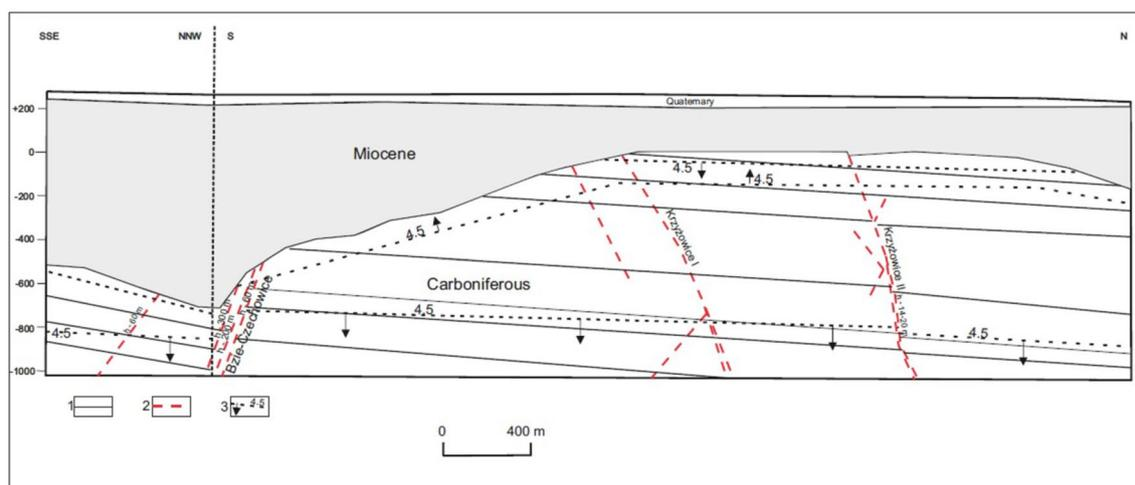
**Fig. 3** The cross-section across the Pniówek Mine, 1—the more important coal seams, 2—fault with throw size  $h$ , 3—line of methane content 4.5 m<sup>3</sup>/t coal<sup>daf</sup>, increase in methane content in the direction of the arrow
