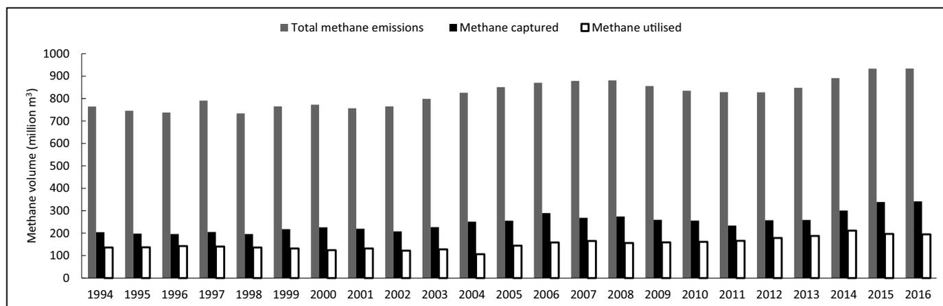
Fig. 11. Total (absolute) methane emissions, methane captured and utilised in the USCB in 1994–2016.
