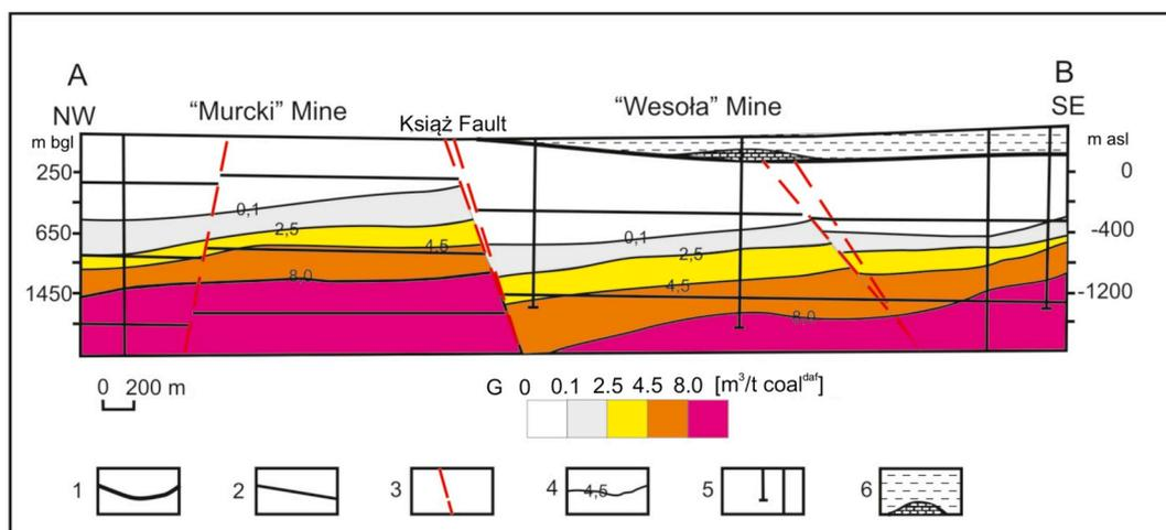
Fig. 7. Cross-section of region 1. The degassed zone ( $G < 4.5 \text{ m}^3/\text{t coal}^{\text{daf}}$ ) reaches a depth of 600–1400 m below ground level. The methane zone ( $G > 4.5 \text{ m}^3/\text{t coal}^{\text{daf}}$ ) occurring below that depth is displaced by the Książ fault.
