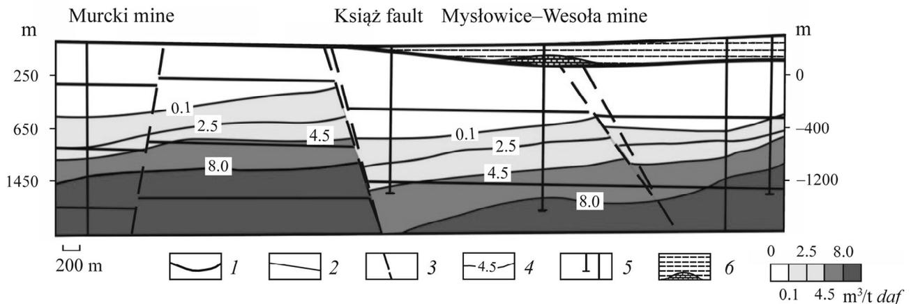
**Fig. 1.** Cross-section of Myslowice–Wesoła mine region: 1—stratigraphic boundary; 2—coal seam; 3—fault zone; 4—line of methane content  $G$  ( $\text{m}^3/\text{t daf}$ ); 5—borehole; 6—Triassic and Miocene strata.
