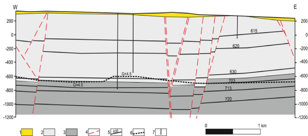
**Figure 7.** Cross-section across the Rydułtowy coal deposit (modified after Rydułtowy mine archive materials): 1—overburden, 2—Poruba layers, 3—Jaklovec layers, 4—fault, 5—coal seam, 6—top of the methane zone with  $G > 4.5 \text{ m}^3/\text{t}$  coal daf, 7—shaft.
