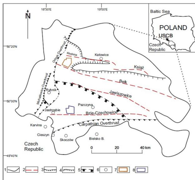
**Fig. 1** Map of the Upper Silesian Coal Basin (modified after Kędzior 2012) 1—the boundaries of the Polish part of the USCB, 2—important fault zones, 3—overthrusts, 4—the range of the continuous Miocene cover, 5—the range of the secondary methane zone (ticks point the direction inside the areas of ranges), 6—important cities, 7—the Budryk mine boundary, 8—the Pniówek mine boundary
