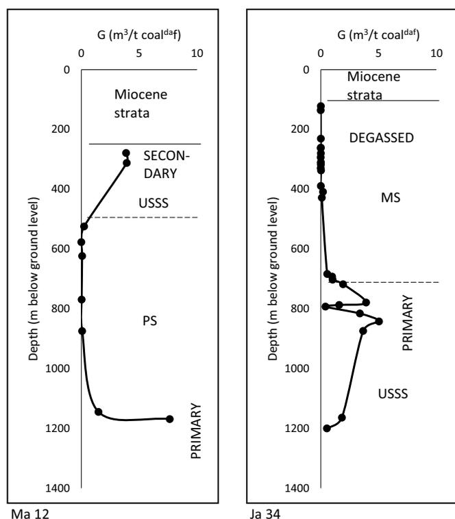
Fig. 4. Depth distribution of methane content (G) in selected boreholes in relation to stratigraphy in region 3.
