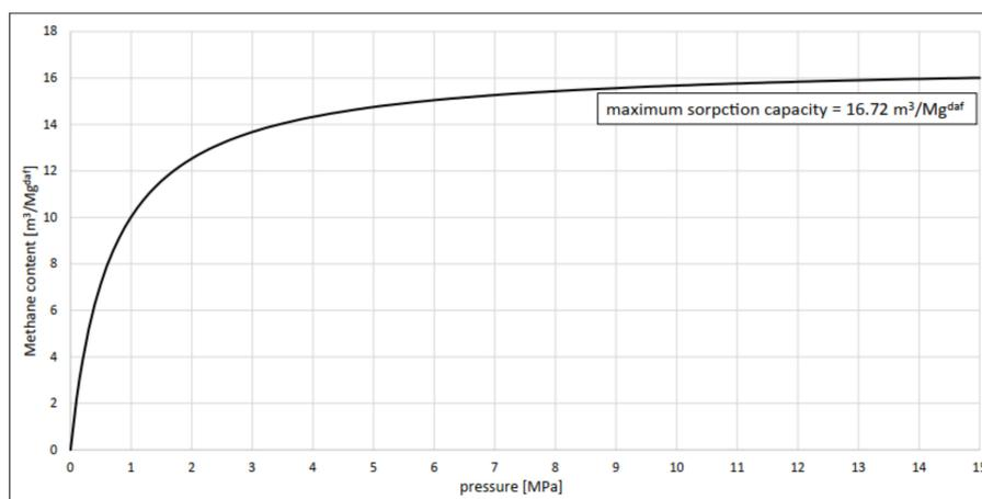
**Figure 4.** Langmuir sorption capacity of the coal from the Rydułtowy mine, taken from the depth of 1000 m.
