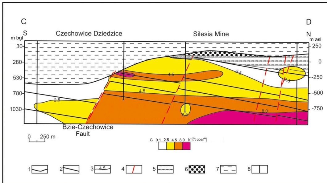
**Fig. 8.** Cross-section of region 2. The methane zone ( $G > 4.5 \text{ m}^3/\text{t coal}^{\text{daf}}$ ) occurs to the north of the Bzie-Czechowice fault, that influences the broken continuity of the zone of methane content. The accumulation of free methane is evident within the erosional elevation of the Carboniferous strata.
