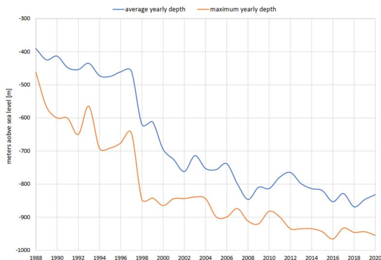
Figure 10. Changes in the average and total depth of the coal output from 1988–2020.
