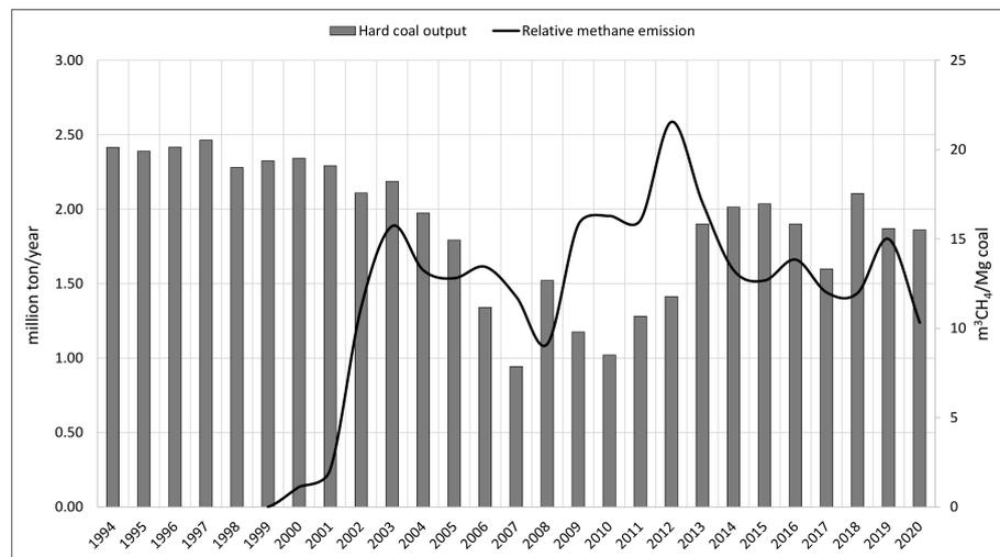
Figure 8. Hard coal output and specific methane emissions from 1994–2020 in the Rydułtowy mine.
