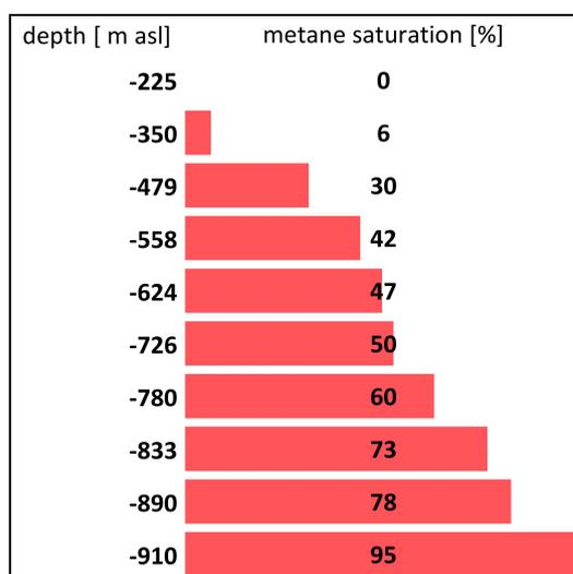
**Figure 5.** Saturation of the coal seams with methane, depending on depth, in the Rydułtowy deposit.
